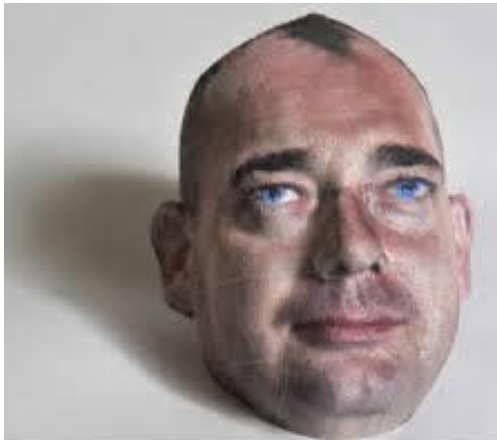
Fig. 5 An Hicor model emerges from the 3D printer as a tough, durable model; no need for infiltration.
